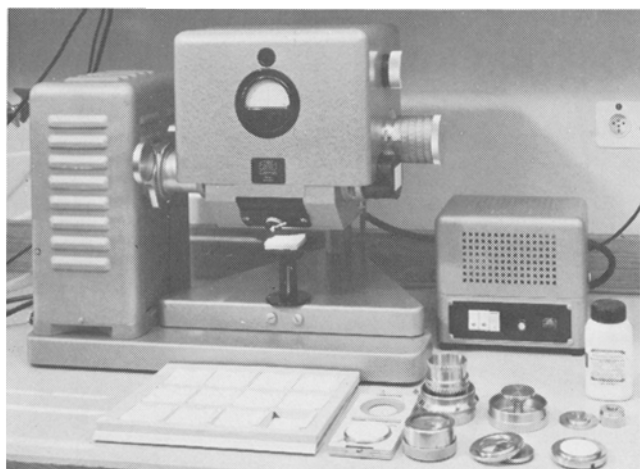
FIG. 3. Elrepho tristimulus filter photometer and xenon lamp 150 W1 + conversion filter for standard illuminant D 6500.
